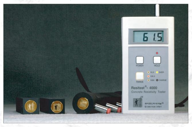
The corrosion of steel in concrete is an electro-chemical process which creates a current flow causing metal to dissolve so that it is possible to assess the probability of reinforcement corrosion by evaluating the electrical resistance of the concrete. The factor is measured in terms of resistivity and expressed in Ohm.
