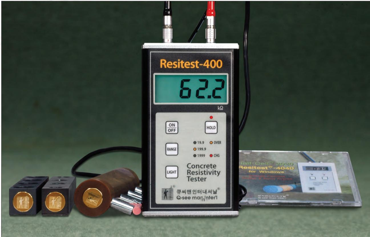
The corrosion of steel in concrete is an electro-chemical process which creates a current flow causing metal to dissolve so that it is possible to assess the probability of reinforcement corrosion by evaluating the electrical resistance of the concrete. The factor is measured in terms of resistivity and expressed in Ohm.
