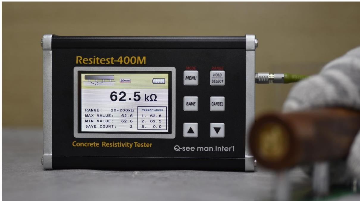
The corrosion of steel in concrete is an electro-chemical process which creates a current flow causing metal to dissolve so that it is possible to assess the probability of reinforcement corrosion by evaluating the electrical resistance of the concrete. The factor is measured in terms of resistivity and expressed in Ohm.
